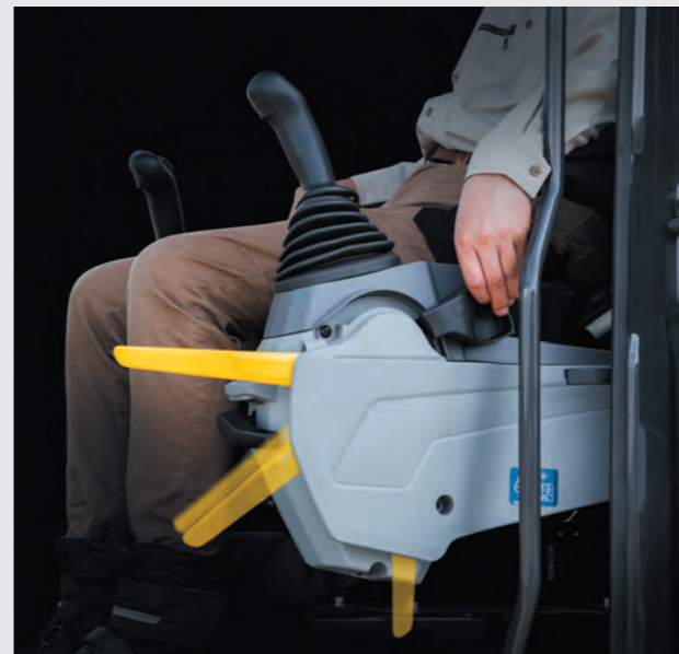
New designed pilot shut-off lever The newly designed pilot shut-off lever allows easier locking and unlocking with wrist operation.
