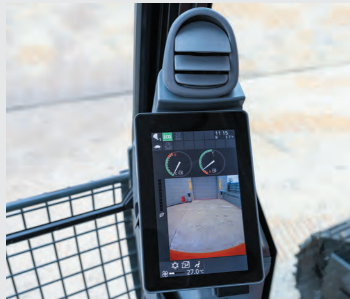
Low-reflective color 8" monitor, 42% larger display compared to ZX-5G series. Easier to view and navigate. Optional USB power supply and Bluetooth® available.
