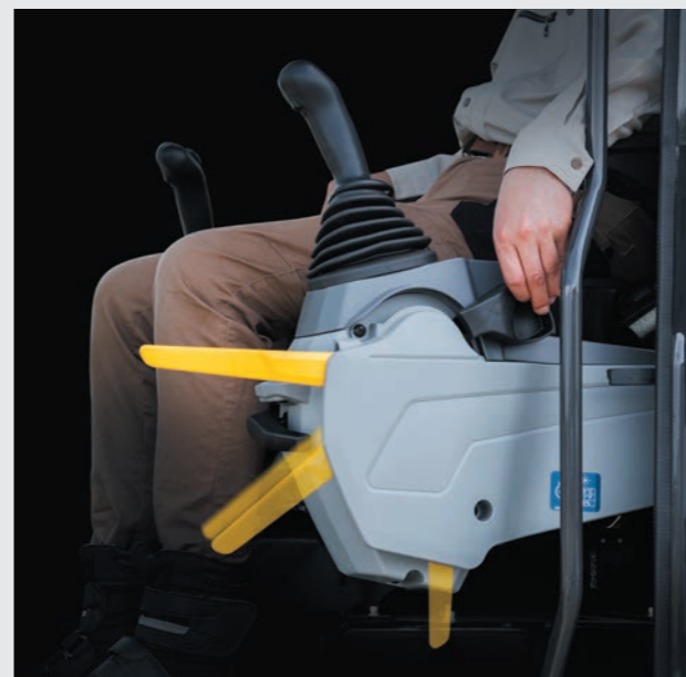
New designed pilot shut-off lever The newly designed pilot shut-off lever allows easier locking and unlocking with wrist operation.
