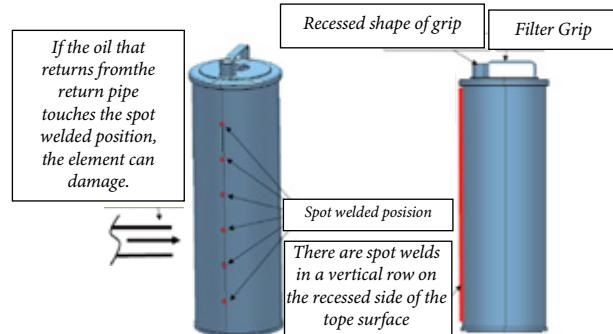
Hydraulic Return Filter installation instructions for each unit model (The following also applies to models equipped with a High Performance Hydraulic Return Filter).
