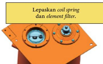
In heavy machinery, proper maintenance of each component can result in optimal equipment performance. Through this news, we inform you that the *Hydraulic Return Filter* on unit models ZX-1~5, ZH200-A/5B, ZXW-1~5 and unit serial numbers ZX-1~5 (16~35 T), ZH200-A / 5B, ZX180W~210W, ZX170W-3~ZX220W-3, and ZX170W~ZX220W-5B may be damaged if the return oil from the return pipe hits the welding point location on the *Hydraulic Return Filter*.
