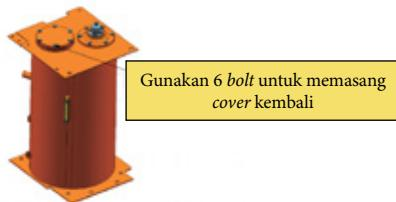
6. Use the 6 bolts that were previously removed to securely attach the cover.
