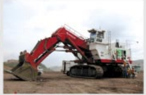
3. HITACHI HYDRAULIC EXCAVATOR EX 3500 (SHOVEL)
