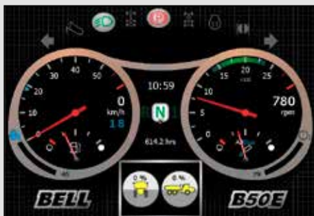
The incorporation of a pitch and roll sensor in the vehicle prevents bin operation if the truck is in an unsafe position.
