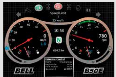
Both operator or site selectable maximum speed control allows the vehicle to automatically decelerate and apply the retarder to prevent onsite speeding.
