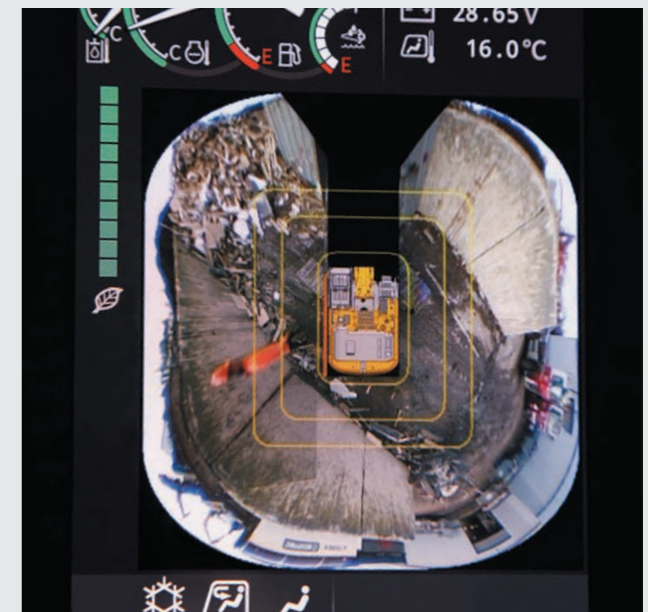
AERIAL ANGLE 270-degree bird's eye-view camera system is available.
